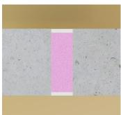
Cross-section of already filled with **Piro Foam 240** and PIROSILICON 240 vertical expansion joint
