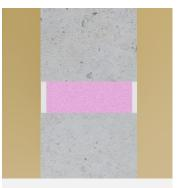
Cross-section of already filled with **Piro Foam 240** and PIROSILICON 240 horizontal expansion joint
