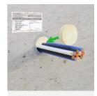
Plug the remaining free space of the duct with the provided plugs. Mark the penetration seal with the attached label, mark **Piro Multitube PM** fireproof intumescent tape on it, enter the date and the name
