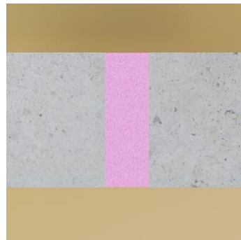
Cross-section of already filled with PIROFOAM 240 vertical expansion joint
