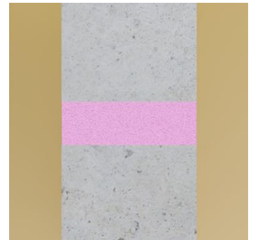
Cross-section of already filled with PIROFOAM 240 horizontal expansion joint
