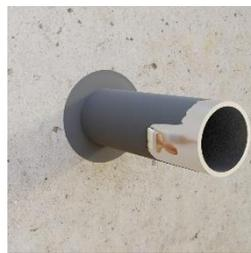
Apply **PiroCoat I** on the pipe so that a ring with a width of min. 500 mm and a thickness of min. 1.2 mm is created
